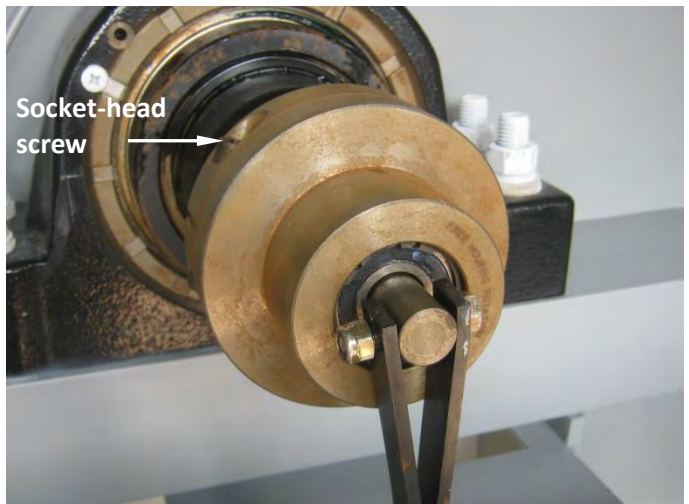
Image 3-9 – Socket-head screw on clutch housing
