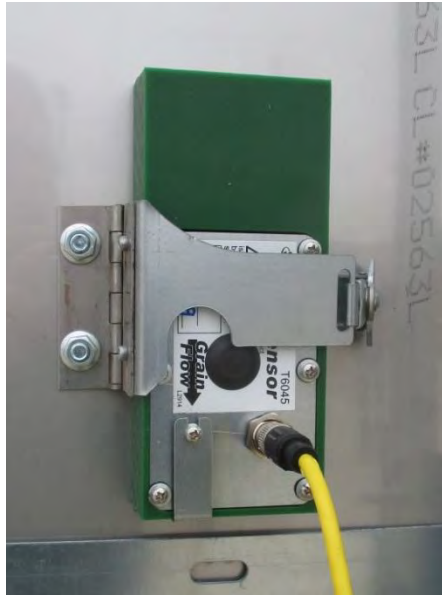
Image 4-9 – Incoming moisture sensor
