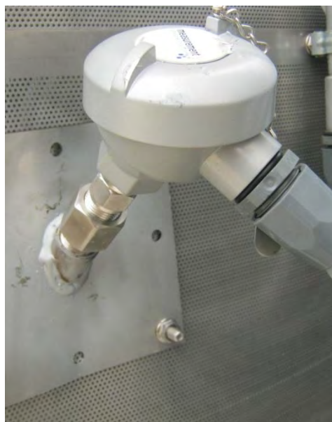
Image 4-12 – Single-point grain column temperature sensor
