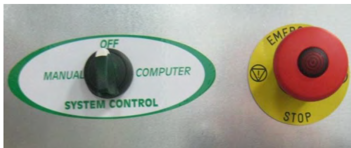
Image 2-1 – System Control switch, Emergency Stop button
