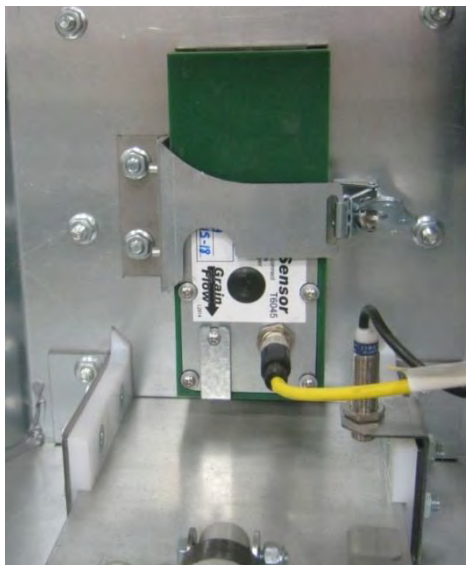
Image 4-10 – Discharge moisture sensor
