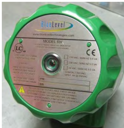
Images 4-2 & 4-3 – Rotary fill switch, fill sensor
