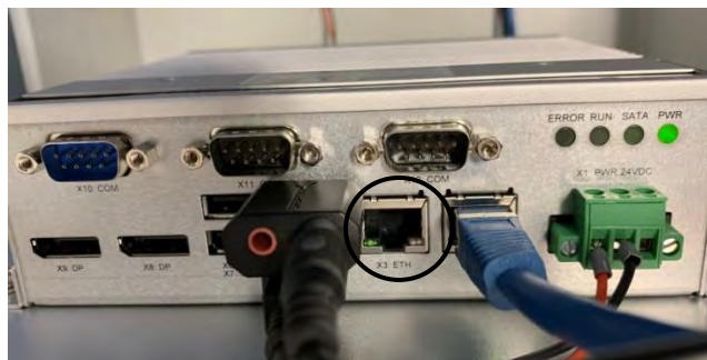
X3 Ethernet port (circled) in touch panel box
