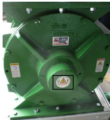
Image 11 – Airlock rotation tag location
