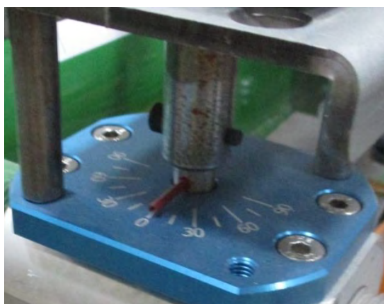
Image 9 –Dynamic bleed valve set at 0%
