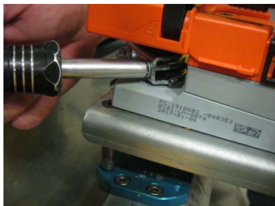
Image 7– Loosening butterfly valve collar
