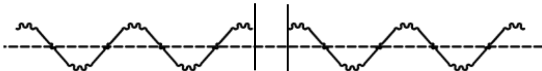
Fig. 11 – Maximum end-to-end gap is 4-11/16" for Hawk Cut flooring
