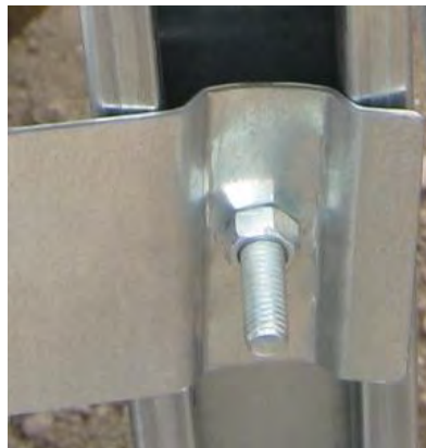
Image 2 – Ladder bracket after attachment to ladder
