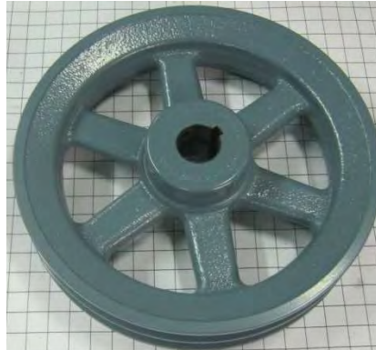
J0365 – PULLEY, 9" OD, 1" ID, DBL B GRV, W/ KEYWAY (8.75" OD, 8.4" PD)
