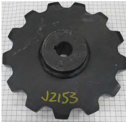
J2153 – SPROCKET, 81X, 13-TOOTH, 1-7/16" BORE
